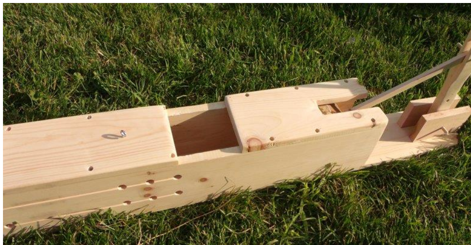
FIGURE 12 DEVICE TO MAKE BALES WITH ONLY MANUAL LABOUR
