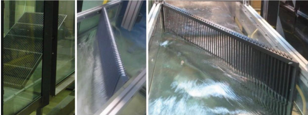
Figure 24. Inclined rack, angled rack with perpendicular bars and angled rack with streamwise bars investigated in laboratory conditions (Raynal, Chatellier, Courret, Larinier, & David, 2015)
