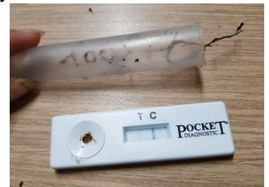
Figure 23: Example of biased results obtained with the Pocket diagnostic on-site tests: here, the 100% infected modality has showed a negative result for Phytophthora sp. while it was well-infected. (HAMEAU, 2019)
