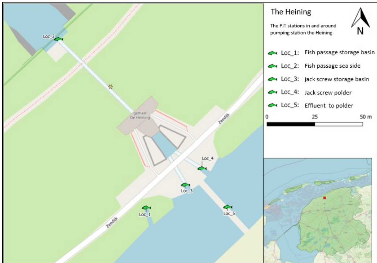
Figure 2.2: Schematic illustration of fish passages in the Heining and the fish passage that forms the connection between the polder and the storage basin. Using a lure flow, fish are lured from the sea to a collection tank (Loc_2). There is a waiting room where the fish gather. After a while, the tank closes and the water flows in free fall to the storage basin (Loc_1). Via fish-friendly jack screw pumps, the fish can migrate back to the sea (Loc_3 and Loc_4). Furthermore, there is a fish passage that forms the connection between the storage basin and the polder (Loc_5).
