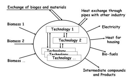
Fig. 3. Schematic representation of an ECP
