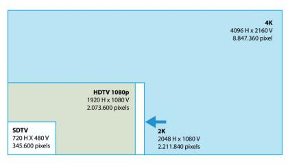
Fig. 1. 4K resolution in comparison to other resolutions.
