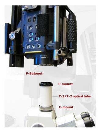
Fig. 3. Optical tube with F-mount and C-mount; the RED ONE video camera with the Nikon F-bayonet.
