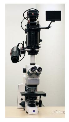
Fig. 2. The RED ONE video camera connected to the microscope.
