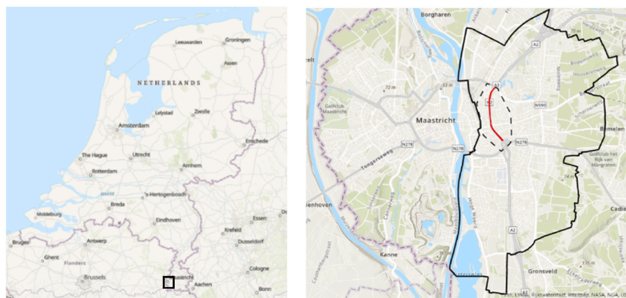
Fig. 1. Left: Location of the city of Maastricht, in the south of The Netherlands; Right: East Maastricht area in black, with reconstructed area in dashed line and in red the highway section that was tunneled.
