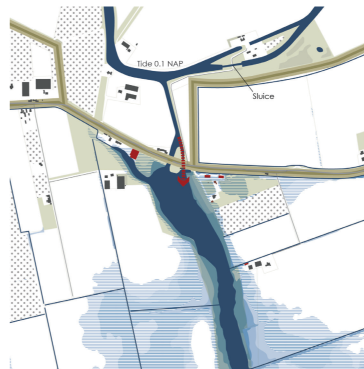
When the water can flow freely, with high tide, the land is slowly flooded.
