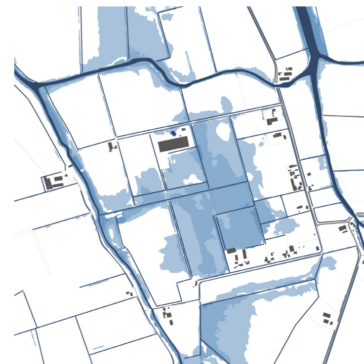
With low tide the land is dry. In the lowest part, water stays and new ponds are formed. This cycle repeat itself on daily basis. In time, the landscape changes. New water channels carved out and other areas become permanent dry because of deposition of sediment. Nature will settle and it become a real estuarium.
