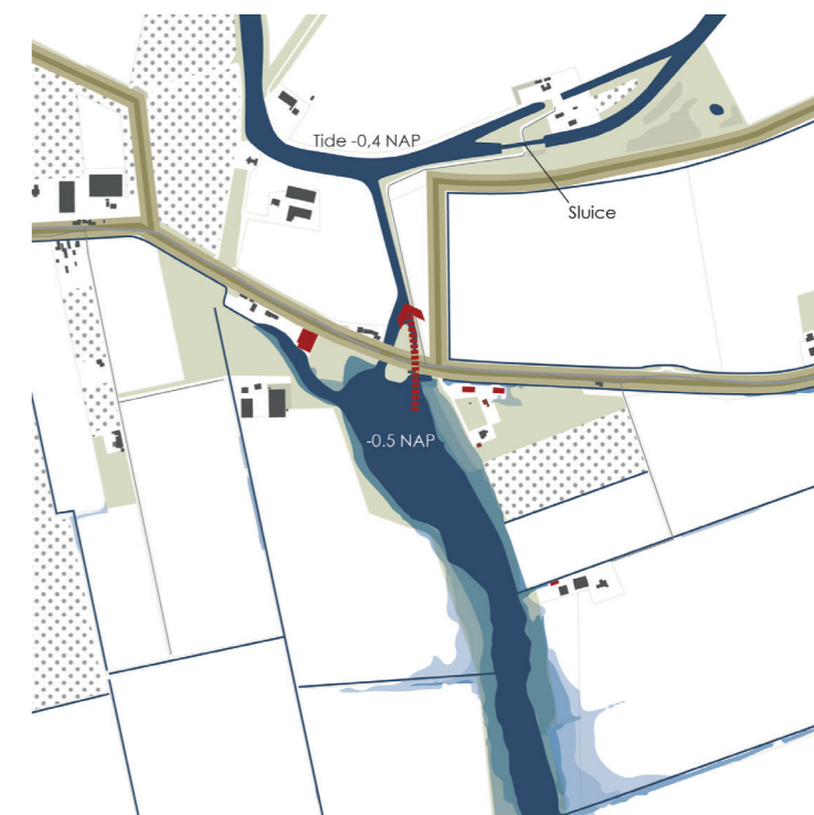
With low tide, the water exists to the vliet and the land become dry.
