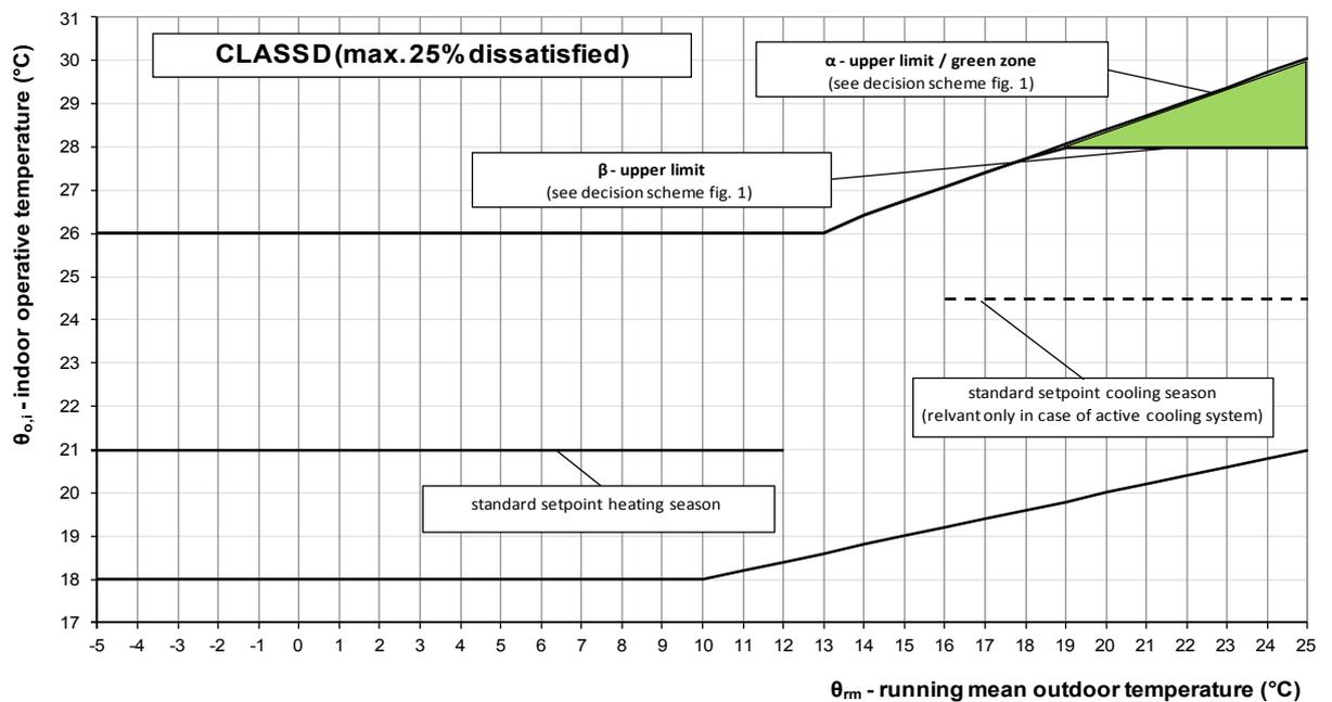
Figure 5. Class D requirements in ISSO 74:2014 for the operative temperature indoors in relation to the running mean outdoor temperature
