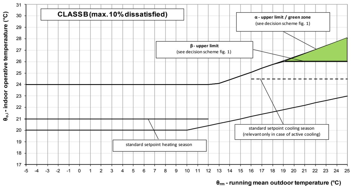
Figure 3. Class B requirements in ISSO 74:2014 for the operative temperature indoors in relation to the running mean outdoor temperature
