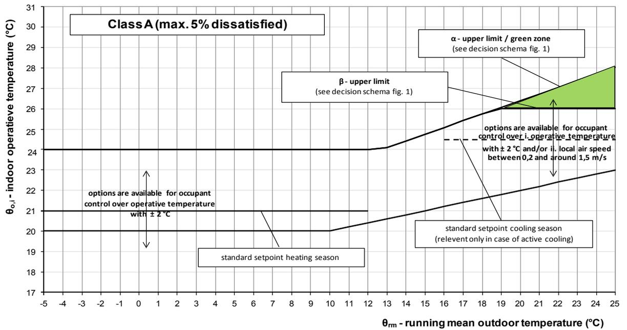
Figure 2. Class A requirements in ISSO 74:2014 for the operative temperature indoors in relation to the running mean outdoor temperature
