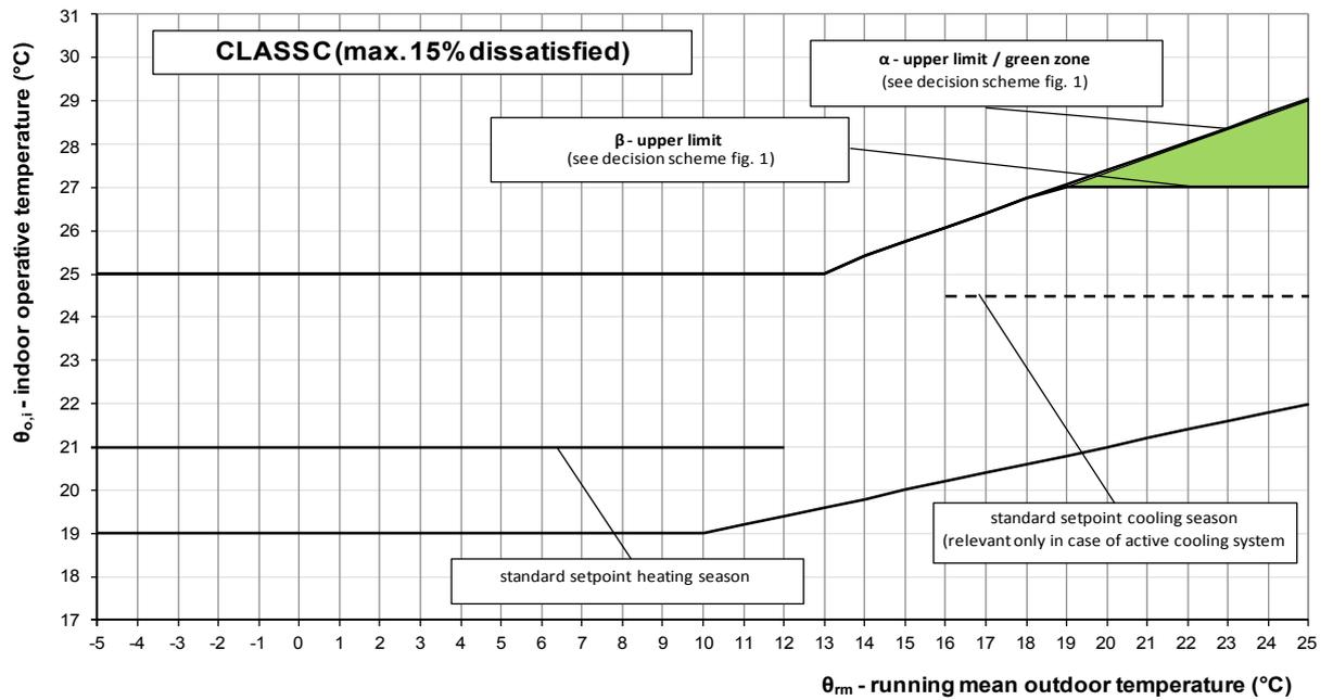
Figure 4. Class C requirements in ISSO 74:2014 for the operative temperature indoors in relation to the running mean outdoor temperature
