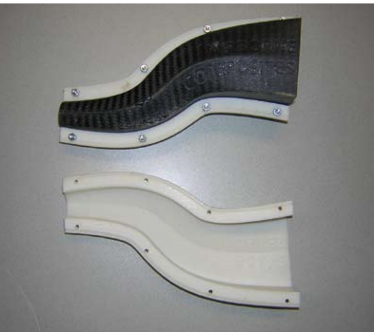
Figure 8. The polycarbonat mould produced with RM, for manufacturing complex-shaped composite products.
