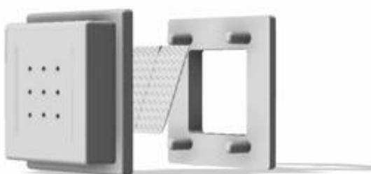
Image 6: 3D exploded view model of the filter inspired by Manta Ray
