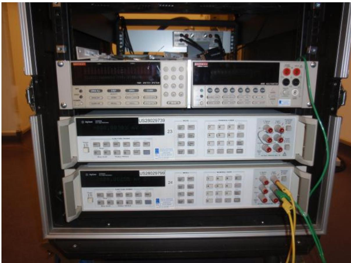
Figure 32: 19" rack containing: switch system (top, left), Keithley 2001 DMM (top, right) and two Agilent 3458A opt 002 DMMs (center and bottom). In the background, the rear panel of the equipment interface box is also seen.
