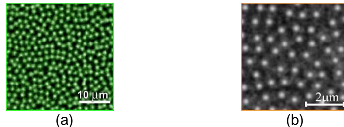
Figure 9. (a) Magneto-optical, (b) magnetic force microscope, imaged vortices in a type II superconductor where bright dots are high flux densities at the superconductor surface, source: ( http://www.mn.uio.no/fysikk/english/research/groups/amks/superconductivity/vortex/index.html ).
