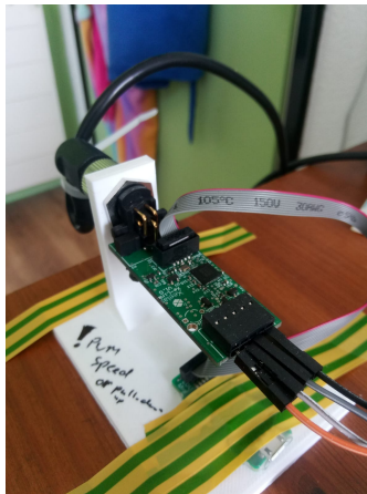
Figure 23 – Result of soldered PCB in 3D printed holder
