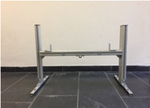
Figure A.16: Support system 1 of the higher part, front view
