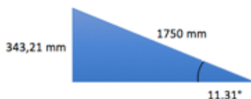
Figure 9.11: Indication of the maximum height of the support construction with an inclination of 20%.
