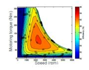
From: Performance/cost comparison of induction-motor & permanent-magnet-motor in a hybrid electric car. Malcolm Burwell International Copper Association
