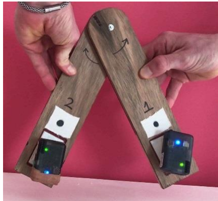
Figure 12, Joint board with markers for Kinovea tracking, the joint's screw is used as the third marker.
