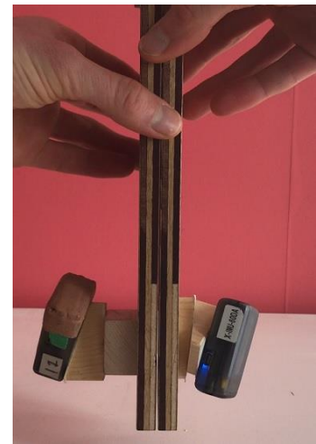
Figure 9, Parallel segments of the hinge joint-model before hitting the model to a flat surface, used to create an accelerometer peak.
