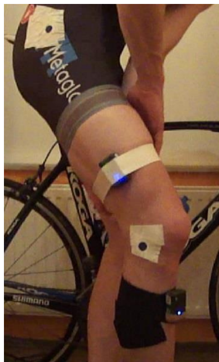
Figure 13, IMU placement at the bike test. IMU1 is placed lateral/distal on the thigh and IMU2 is placed frontal/proximal on the tibia.
