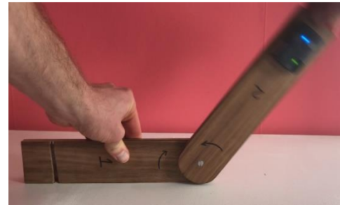
Figure 11, Generation of angular rotations around the hinge joint by turning one of the two segments.
