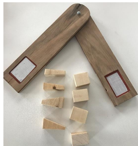
Figure 7, The joint-model with a hinge-joint. The spacers can be used for arbitrary positioning the IMU's to unknown placements on each segment.
