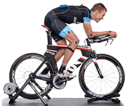
Figure 1, Fixed bike position for measuring the cyclists kinematic movements with a system from Retul. Source: http://motionfit.net/bike-fit/
