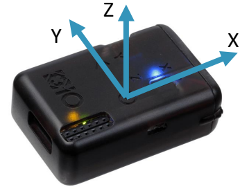
Figure 5, IO x-IMU with case and its representing local coordinate system.
