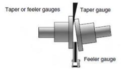
Figure 5-14: Feeler gauge measurement
