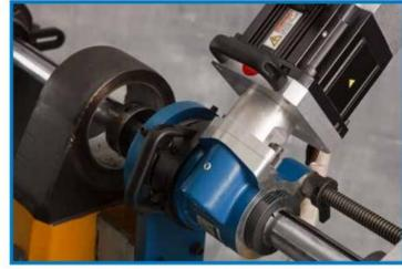
Patented heavy-duty spherical bearing mounts ensure rigid attachment to the work piece, for more effective machining.
