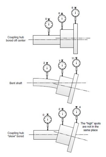
Figure 5-6: Shaft deflection measurement
