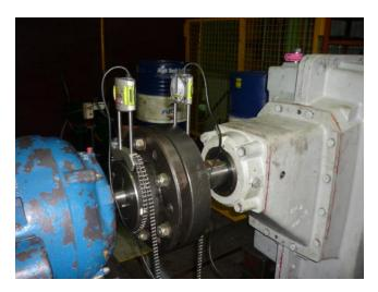
Figure 5-16: Laser alignment set-up
