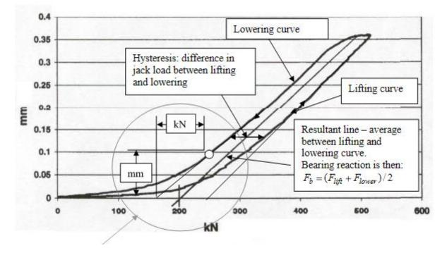
Figure 5-13: Jack-up curve (ABS, GUIDANCE NOTES ON PROPULSION SHAFTING ALIGNMENT, 2006)
