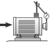
Figure 5-4: Run-out measurement set up
