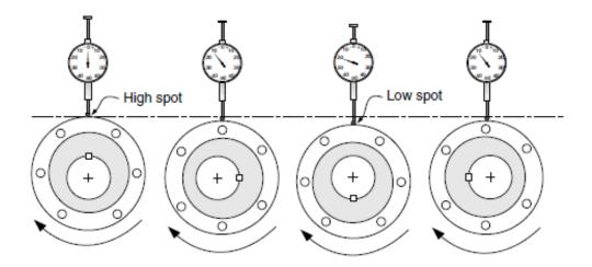
Figure 5-5: Visual representation of run-out
