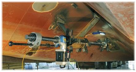
Figure 5-20: Line boring equipment (Redd, 2010)
