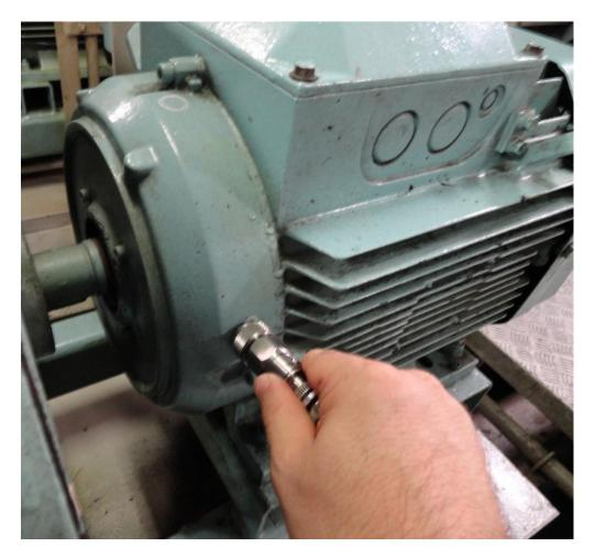
Figure 5-8: Vibration measurement (Staykov, Accelerometer mounting, 2014)
