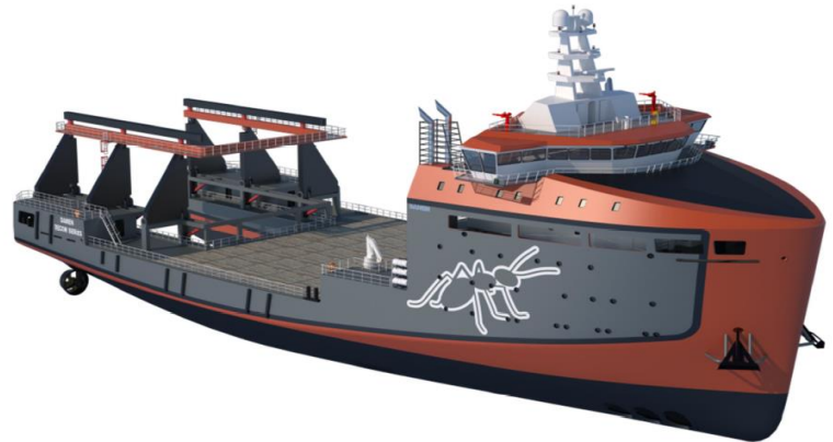
Figure 7 The decommissioning vessel, equipped with lifting frame
