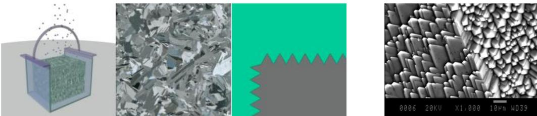
Figure 5: Surface after texturing. From left to right: the wet bench, the silicon surface, the silicon surface schematically and an image of the grain boundaries. (Marstein, Silicon Solar Production, 2012)
