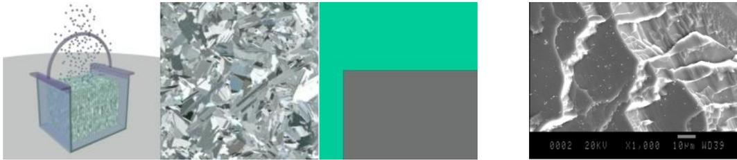
Figure 4: Surface after damage removal. From left to right: the wet bench, the silicon surface, the silicon surface schematically and an image of the grain boundaries. (Marstein, Silicon Solar Production, 2012)
