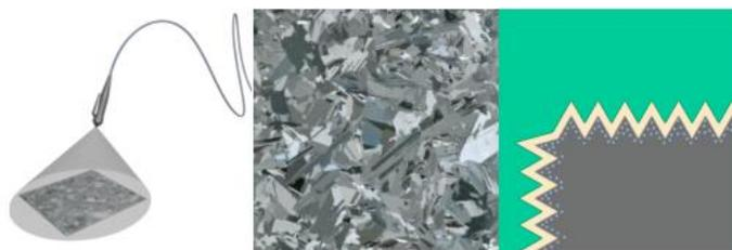
Figure 6: Surface after diffusion. From left to right: adding emitter, the silicon surface and the silicon surface schematically. (Marstein, Silicon Solar Production, 2012)
