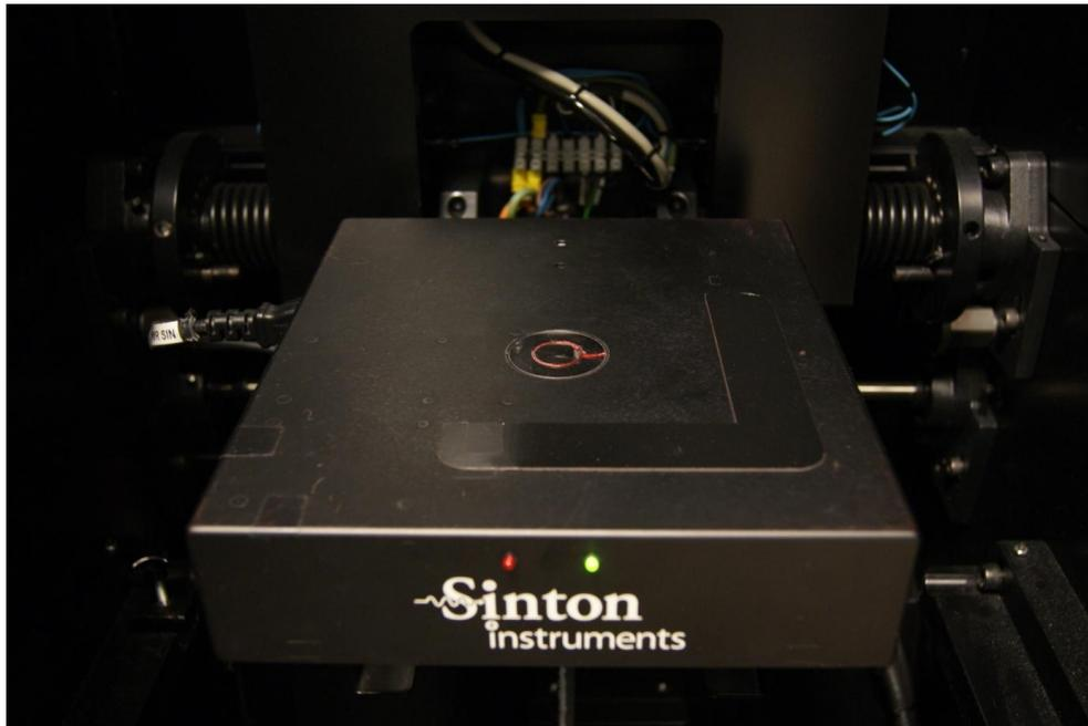
Figure 13: Calibration stage with coil in the middle
