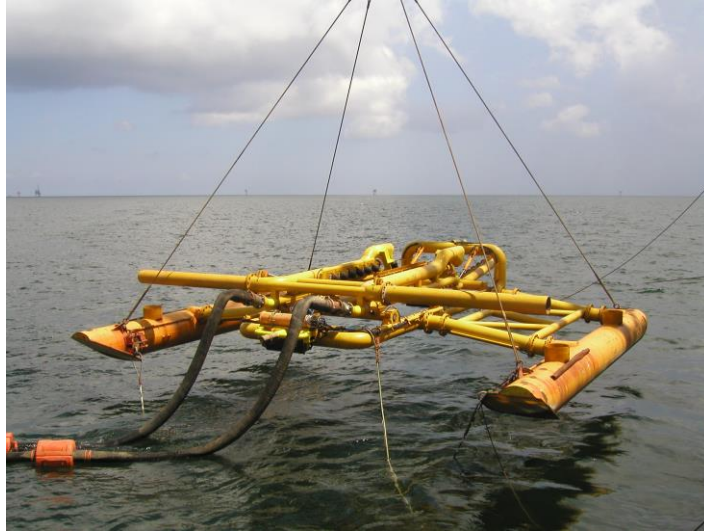
Figure 2.2 Deploying of the old Jet Sled (Allseas, 2016)
