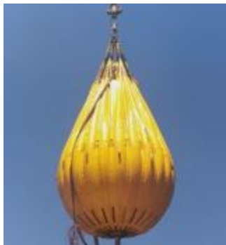
Figure 25, Test load water bag
