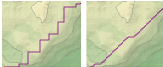
Figure 6.7: Paths with different connectivity. The one on the left has 4-connectivity and the one on the right has 8-connectivity.
