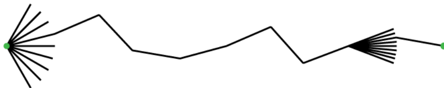
Figure 6.2: Schematic display of the point spread as you approach the endpoint. The fan on the left indicates the selection-angle when starting. The fan on the right indicates the selection-angle near the end of the road.
