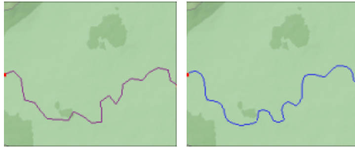
Figure 6.20: Differences in result with post-process smoothing. The left image shows a road without and the right image shows a road with filter applied.
