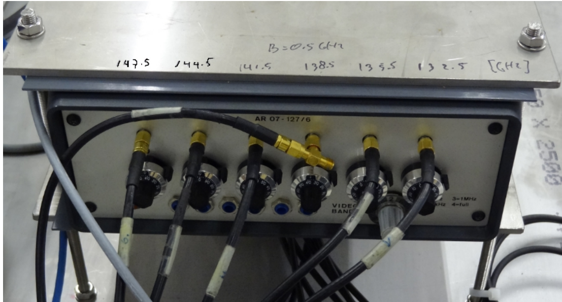
Figure 5.6: Radiometer used for detecting the ECE frequencies. Six channels with different frequencies (channel 1: 132.5 GHz; channel 2: 134.5 GHz; channel 3: 138.5 GHz; channel 4: 141.5 GHz; channel 5: 144.5 GHz; channel 6: 147.5 GHz)
