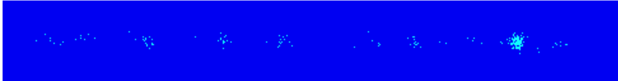
Figure 10. A cosmic ray as measured with the Quad GridPix detector using a generic drifter and a homogenous electric field. The gas mixture consist of 5% isobutane and 95% argon. Showing the detector's x y plane. The color indicates the drift time which is equal for the whole track typical for cosmic rays (in principle, but depending on the test setup). Note the \delta -rays.
