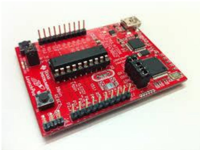
Figure 9 - TI LaunchPad with MSP430G2553 microprocessor with 16 MHz frequency, 16KB flash and 8channel 10-bit ADC.
