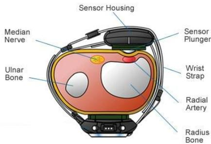
Figure 8: Possible configuration of Applanation tonometry used in the BPro [67]
