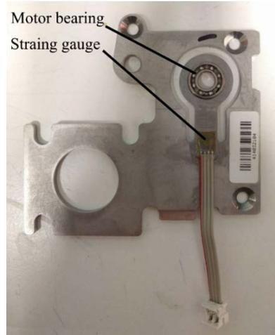
**Figure 4: Motor baseplate containing the motor bearing and the strain gauge used to obtain pressure values. The friction counteracting force exerted by the motor, causes strain on the metal around the motor bearings. This causes the metal, at the location of the strain gauge, to bend slightly. This bending is calibrated to pressure values at the syringe plunger. [31]**
