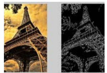
Figure 3: edge detection on a picture [34], with the original picture on the left and the edge detected picture on the right
