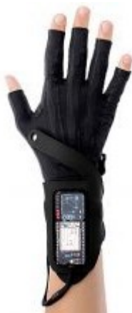
Figure 5: IMU sensor glove by ML.MU, which contains one imu and several pressure sensors [33]
