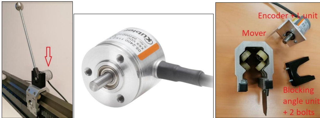
Figure 26: Pendulum encoder [17] and mounting units
