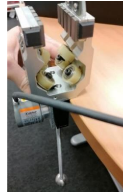
Figure 34: Checking the setpoint value with the earth gravity
