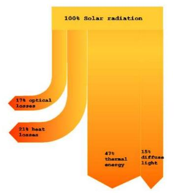
Fig. 2. Overview of the energy flows in a Fresnel greenhouse (Sankey-diagram).
