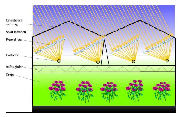
Fig. 1. Impression of a Fresnel greenhouse with tracking Fresnel lenses between the trellis girder and the gutter.
