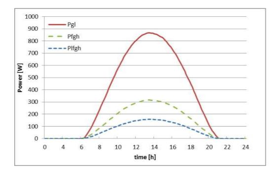
Fig. 4. Calculated results of the global radiation  $(P_{gl})$  on a clear day May 3 the Netherlands (Wageningen), the heat load inside a Fresnel greenhouse  $(P_{fgh})$  and the corresponding cooling effect by transpiration of tomato crops  $(P_{lfgh})$ .
