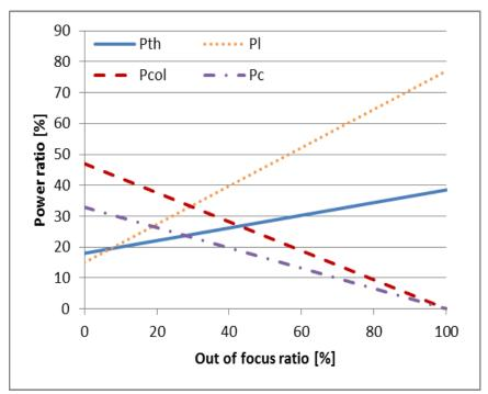
Fig. 5. Effects of different out of focus ratios of the collector on the energy flows
