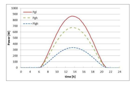
Fig. 3. Calculated results of the global radiation  $(P_{gl})$  on a clear day May 3 the Netherlands (Wageningen), the heat load inside the greenhouse  $(P_{gh})$  and the corresponding cooling effect by transpiration of tomato crops  $(P_{lgh})$ .
