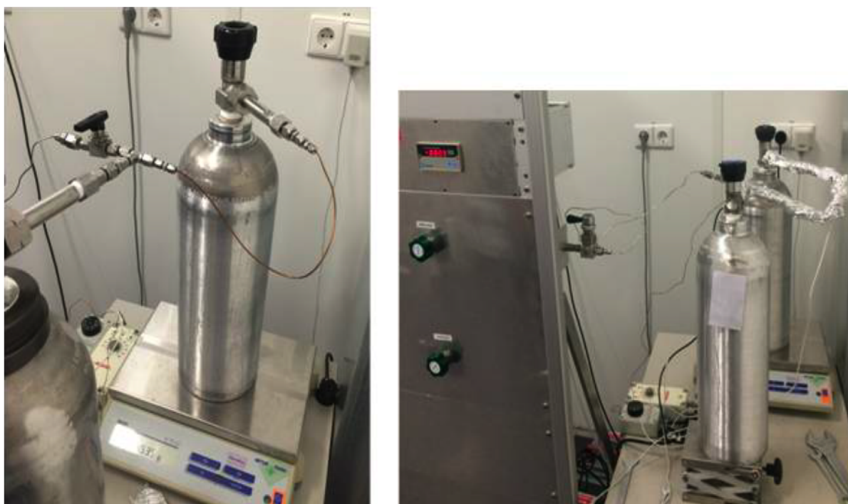
Figure 3.5: Picture of the set-up (left), including heating of the tubing (right).
