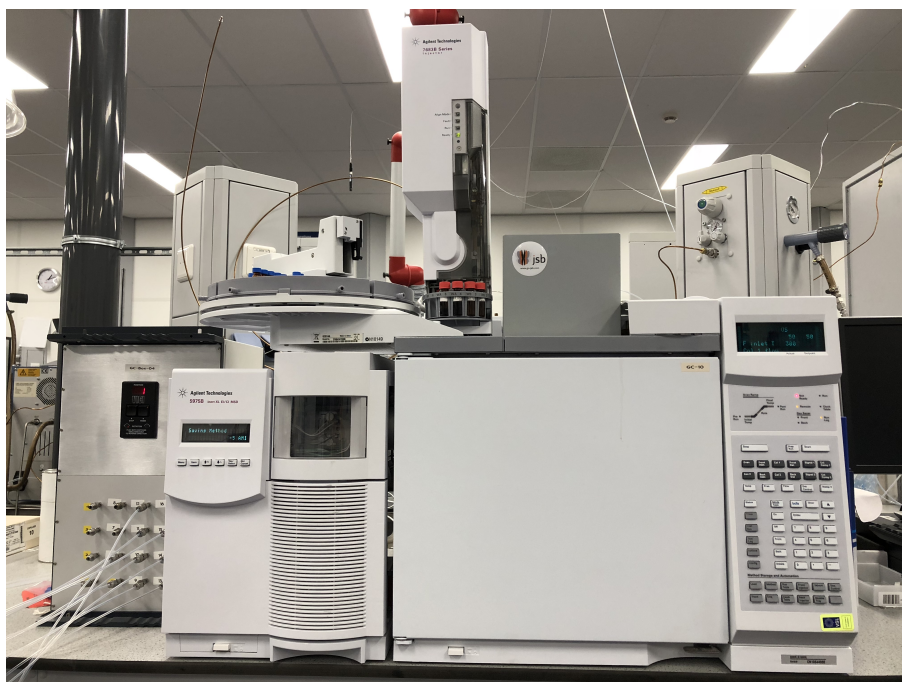
Figure 3.6: The Agilent 5975B GC with gas autosampler and pressure controlling device used for the analyses.
