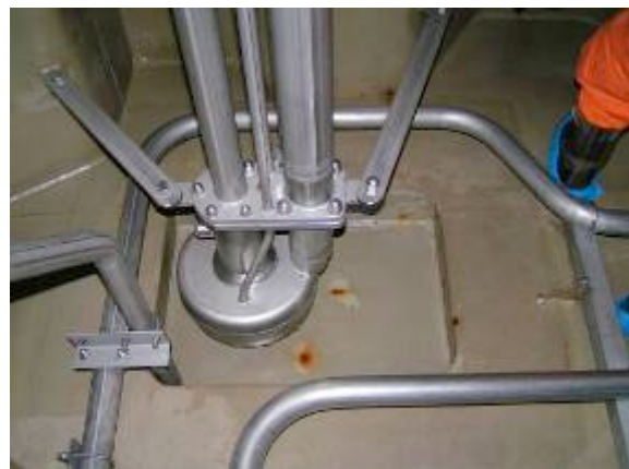
Tank of a chemical tanker (photo 1) each tank is fitted with a submersible pump (photo 2)
