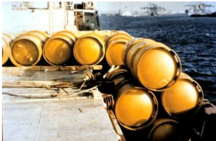
Photo 7 Unstable deck cargo of chlorine cylinders
