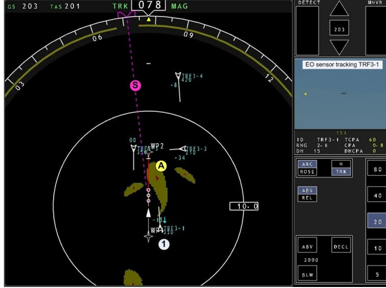
Figure 3: Plan-view conflict probe display, depicting an example scenario with four other aircraft and an impending Loss of Separation.
