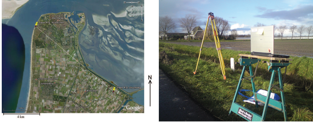
Figure 1: Signals were recorded simultaneously 9 December 2008, at two stations equipped with software receivers and located in the surroundings Den Helder, The Netherlands. Left: map (Google) indicating the baseline location, where the yellow pins indicate the two stations. Right: software receiver recording set-up at the Stoomweg station where the small antenna is positioned on top of the tripod.
