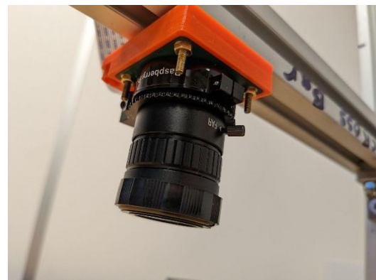
Figure 25 3D Printed Camera mount with the Pi HQ Camera
