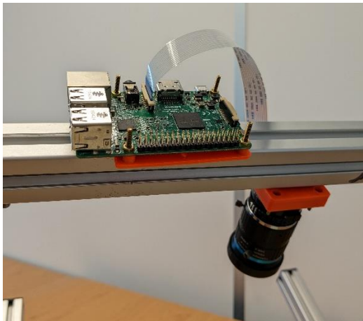
Figure 26 Raspberry Pi and Camera Mounted
