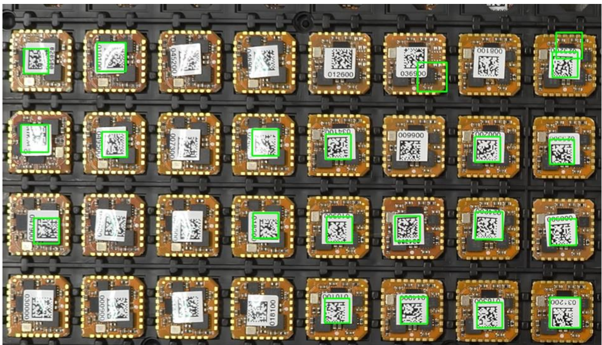
Figure 66 Tray with sensors showing object detection and image glare.
