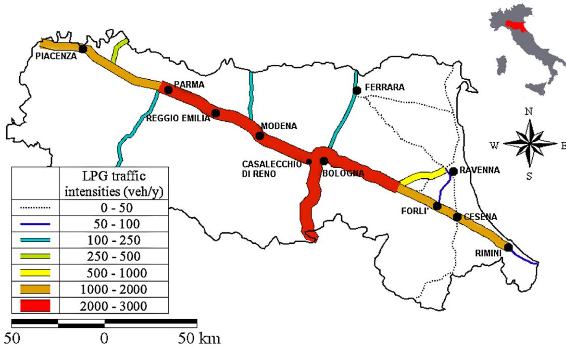
Fig. 6. Case-study 2: the motorway network and the LPG traffic intensity distribution.
