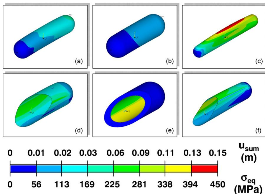
**Fig. 2.** Deformation maps ( $u_{\text{sum}}$ , in m) and stress intensity distributions ( $\sigma_{\text{eq}}$ , in MPa) for tests BF1 (a and d), BF2 (b and e) and BF3 (c and f), calculated on the basis of thermal simulations reported in Fig. 1.
