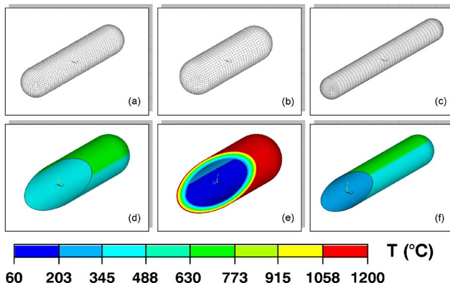
**Fig. 1.** Details on the geometry and mesh used for the validation of FEM with experimental results for tests: (a) BF1–4 m<sup>3</sup> tank; (b) BF2–4.85 m<sup>3</sup> tank; (c) BF3–120 m<sup>3</sup> tank. Temperature maps ( $T$ , in °C) calculated at the end of simulation runs are also reported: (d) test BF1; (e) test BF2; (f) test BF3.
