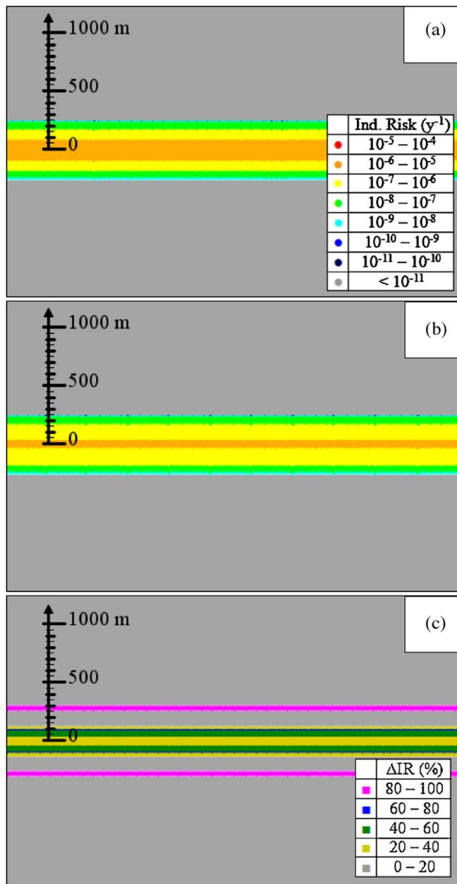
Fig. 8. Case-study 1: (a) individual risk distribution for non-coated tanks; (b) individual risk distribution for coated tanks; (c) percentage reduction in individual risk  $\Delta IR$  due to coating.
