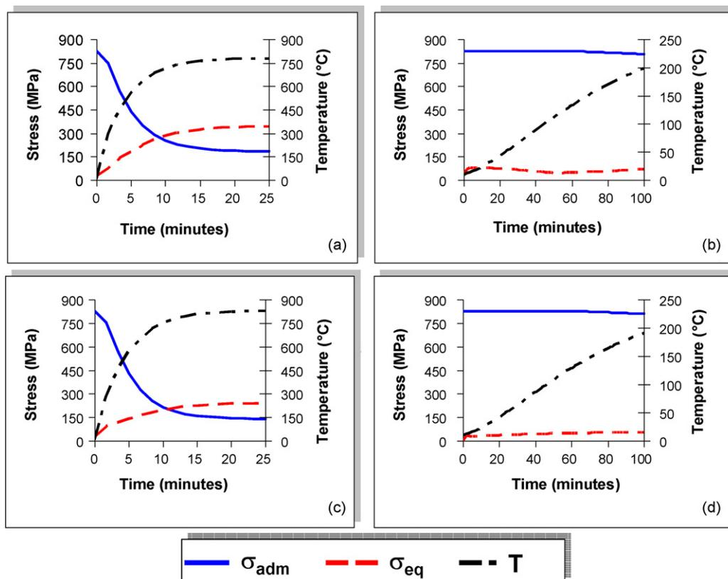
**Fig. 4.** Real scale simulations: dynamic behaviour of maximum allowable stress ( $\sigma_{adm}$ ), stress intensity ( $\sigma_{eq}$ ) and temperature ( $T$ ) in the more critical points. Results are referred to (a) unprotected and (b) protected road tanker; (c) unprotected and (d) protected tank wagon. Stress in MPa, Temperature in °C.
