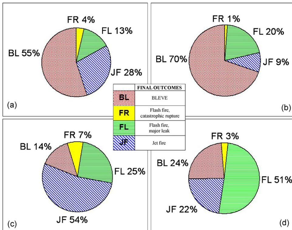
Fig. 11. Case-study 1: contribution of the final outcomes to Expectation Value *EV* (a) non-coated tankers and (c) coated tankers; and to Risk Integral *RI* (b) non-coated tankers and (d) coated tankers.
