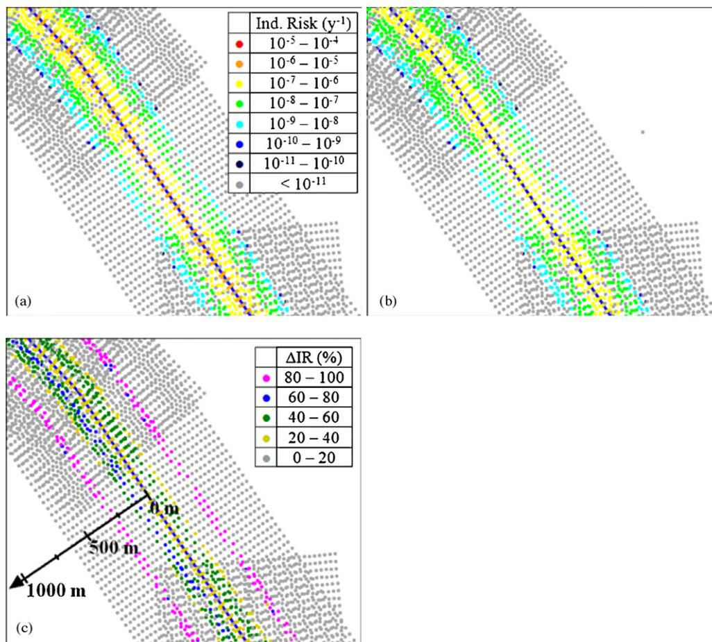
Fig. 14. Case-study 3: Individual risk calculations. (a)  $IR$  for non-coated tankers; (b)  $IR$  for coated tankers; (c) differences in individual risk values are also reported (c)  $\Delta IR$  plot.
