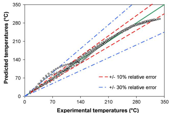
**Fig. 3.** Parity plot reporting the comparison between the maximum wall temperatures predicted by the model and those reported in several previous experimental studies [34,35,43].
