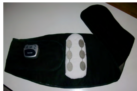
Figure 9: Medical back belt with integrated neuromuscular electrical stimulation
