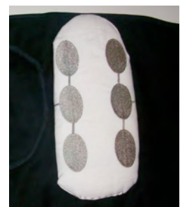
Figure 7: Orthopaedic pad with textile electrodes
