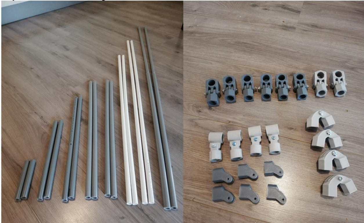
Figure 3.5 The PVC pipes and final set of 3D printed and assembled joints for the wing frame
