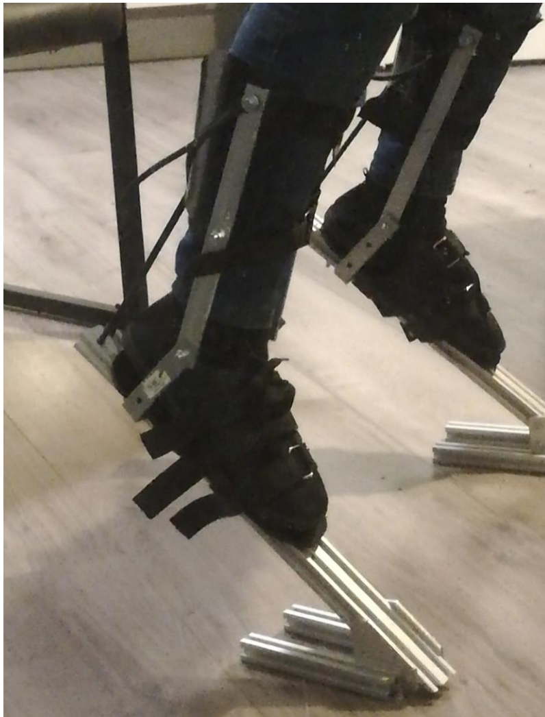
Figure 3.4 The aluminum toe walking stilts designed and built for Kerapac
