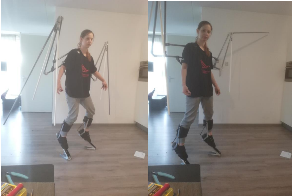
Figure 3.6 The wing frame assembled, folded (right) and extended (left)
