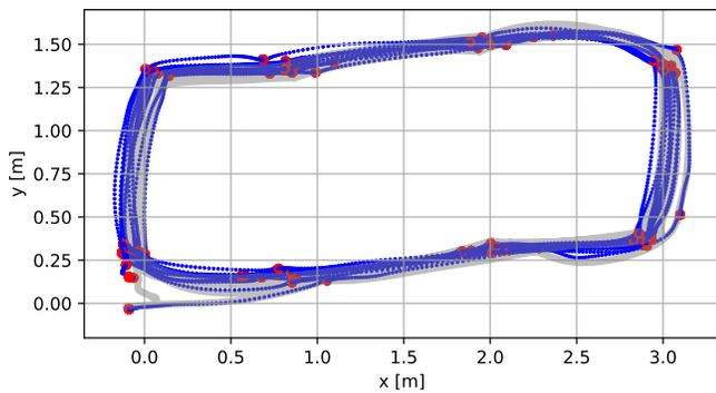
Fig. 3: Reconstruction of an example trajectory. Visible is the planar position estimated with the IMU system (blue dots) and measured with the optical reference system (grey). In addition, ZUPT periods are indicated with red dots.
