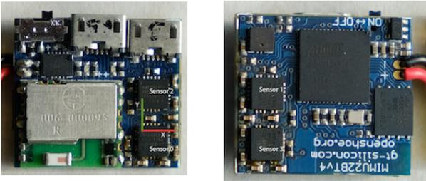
Fig. 1: Top and bottom view of the MIMU22BT. Visible are four Invensens 9205 modules. Sensor 0 is mirrored with sensor 3 and sensor 1 is mirrored with sensor 2. The right-handed coordinate frame of sensor 0 is indicated ( $x$ =red,  $y$ =green). The relative distance between sensor 0 and 2 is 6.3mm.
