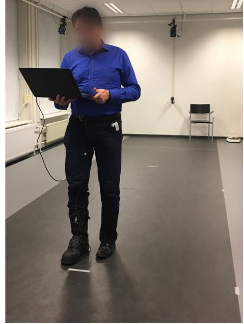
Fig. 2: Subject wearing the firefighter boots with embodied MIMU module. Data is transmitted to a laptop via USB. The trajectory is outlined with white adhesive tape on the floor. In addition, optical markers and cameras of the reference system are visible.
