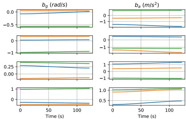
Fig. 5: Estimated sensor biases for each gyroscope (left) and accelerometer (right) pair. For each sensor the x (blue), y (orange) and z value (green) is indicated.
