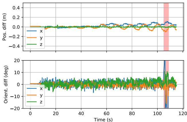
Fig. 4: Differences in the optical and inertial measurement systems. Visible are the position (upper) and orientation (lower) as function of time.
