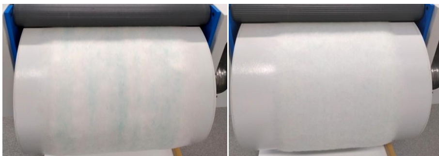
(a) After first carding (b) After second carding Figure 11. Carded web results of the evenness of the blend
