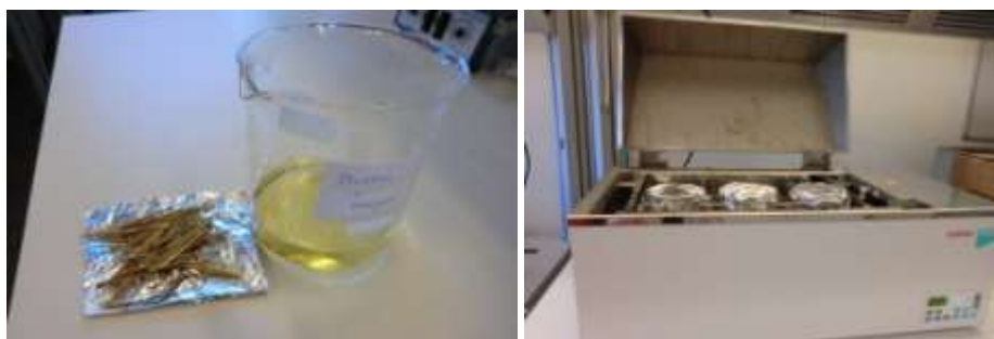
Figure 1: Left - The glass beaker with 0.5M Tris-HCl buffer and untreated chopped flax stems. Right: The water bath at 60°C, where flax retting takes place in closed glass beakers.
