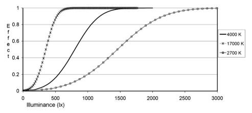
Fig. 3. Hypothesised size of NIF effects of light during daytime for different illuminances at the eye and different colour temperatures. Taken and adapted from Górnicka [30].
