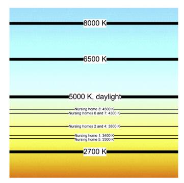
**Fig. 4.** Medians of measured colour temperature in the seven nursing homes compared to the threshold limits of 5000 (daylight); 6500 and 8000 K [26,27] and the common CCT of 2700 K of fluorescent lamps.
