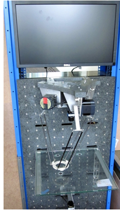
Figure 1.7: An equiplet with a delta-robot frontend
