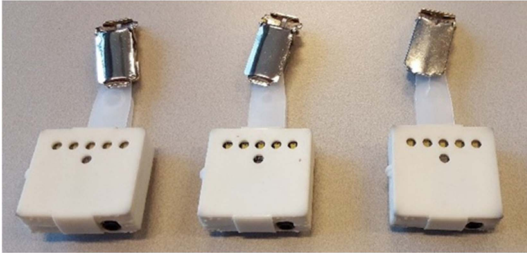
Fig. 8. Portable photometers (Lightlog, developed by G. Martin (2016) [8]).
