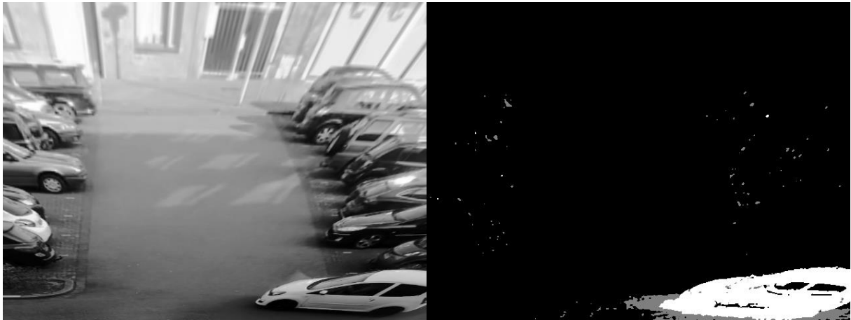
Figure 14: The background segmentation. (left) input image segmented to (right) mask image produces by MOG2. White indicates a moving object. Shades detected in the source are drawn in grey.
