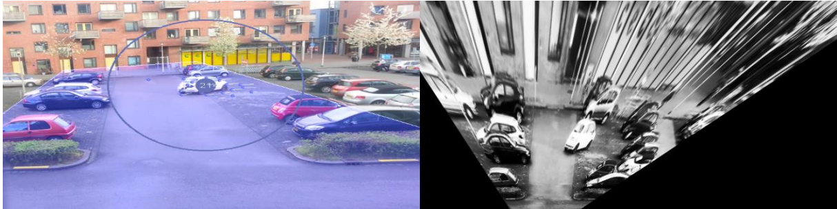
Figure 12: Larger input quadrilateral for a "top view" of the park. The viewing angle of the camera is clearly visible.
