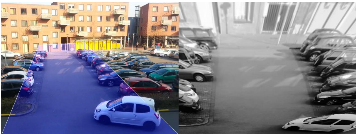
Figure 11: (left) the overlay quadrilateral used for extracting the (right) warped image. Background of the park has less detail than the foreground as seen in this figure.
