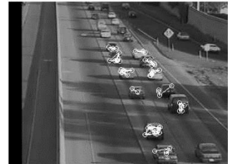
Figure 7: Example of feature points grouped using a Kalman filter (Beymer, McLauchlan, Coifman, & Malik)
