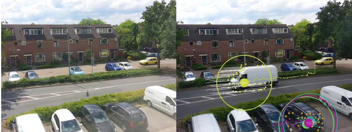
Figure 39: Two frames of fragment 3. (Left) The bright start situation. (Right) the detected van and wrong identified movement in the bottom.
