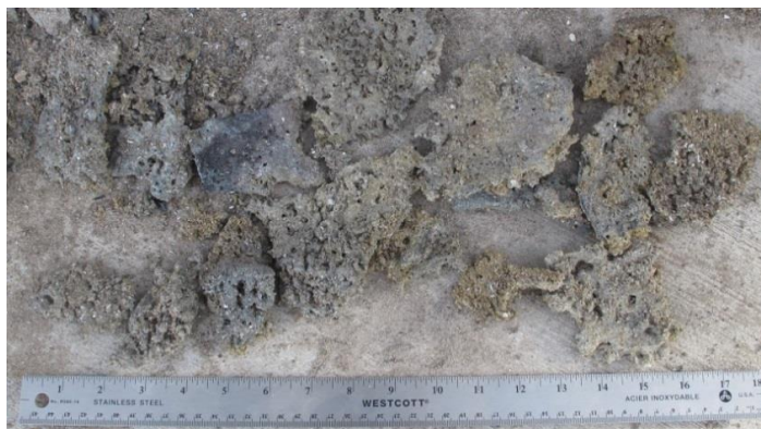
Figure 3.11: Slag build up within the combustion chamber
