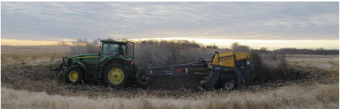
Figure 3.6: The harvesting of WR #2 with the Anderson Biobaler
