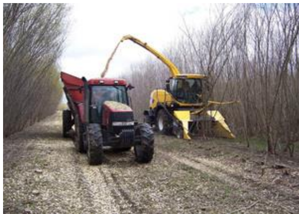
Figure 3.4: A self-propelled harvester
