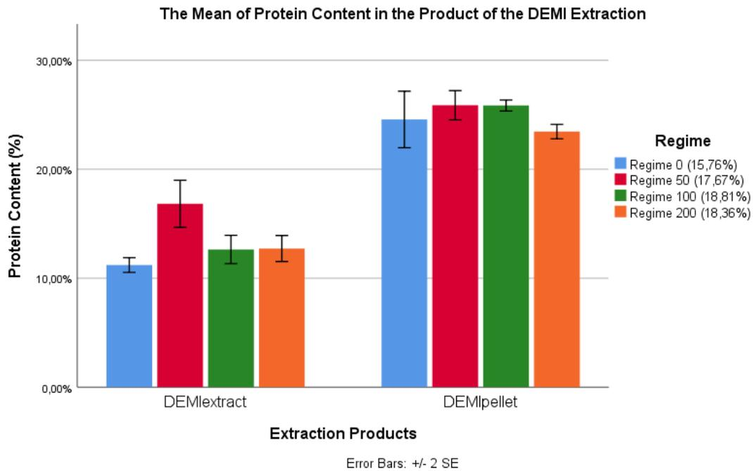
**FIGURE 9:** THE AVERAGE VALUES OF THE PROTEIN CONCENTRATION ON DRY WEIGHT BASIS OF THE DEMINERALIZED WATER EXTRACTION PRODUCTS MEASURED IN EACH SAMPLE (N=3). DIVIDED BY REGIME AND THEIR CORRESPONDING START PROTEIN. THE ERROR-BARS REPRESENT THE STANDARD ERROR.
