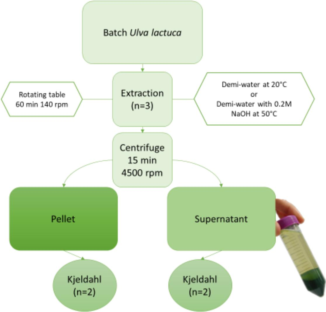
FIGURE 3: SCHEME OF THE EXTRACTION METHOD AND PROTEIN ANALYSIS FROM TOP TO BOTTOM. INCLUDING THE TWO DIFFERENT EXTRACTION METHODS, EITHER DEMINERALIZED WATER AT 20°C OR DEMINERALIZED WATER WITH 0.2 M NAOH AT 50°C.
