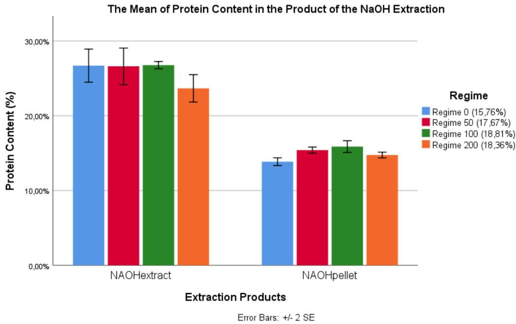
**FIGURE 8:** THE AVERAGE VALUES OF THE PROTEIN CONCENTRATION ON DRY WEIGHT BASIS OF THE NaOH EXTRACTION PRODUCTS MEASURED IN EACH SAMPLE (N=3). DIVIDED BY REGIME AND THEIR CORRESPONDING START PROTEIN. THE ERROR-BARS REPRESENT THE STANDARD ERROR.
