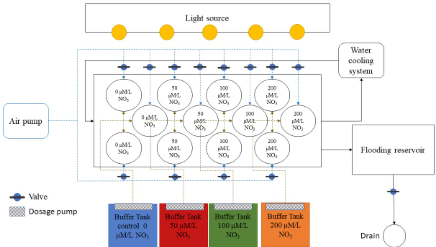
FIGURE 1: EXPERIMENTAL SET -UP SCHEME FOR CULTIVATING *U. LACTUCA*. INCLUDING THE LAYOUT OF THE BUFFER TANKS WITH THE DIFFERENT NITRATE CONCENTRATIONS IN THEIR PLACE WITHIN THE SET-UP AND A LEGEND DEPICTING THE DOSAGE PUMPS AND VALVES.
