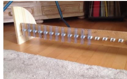
Figure 45: developed construction to measure the water permeability of all samples at once.
