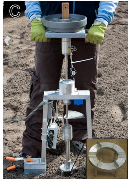
Figure 19: The Shear Vane device in action so weights are applied. (Setterbo et al. 2012 a).
