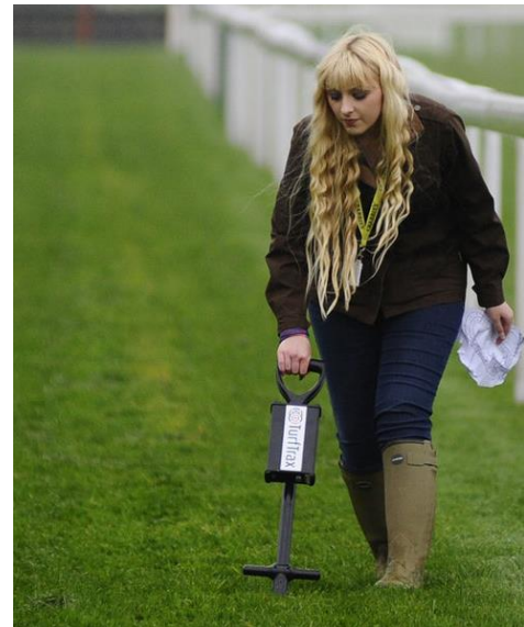
Figure 17: The Going Stick in action (Sky Ltd., (n.d.))
