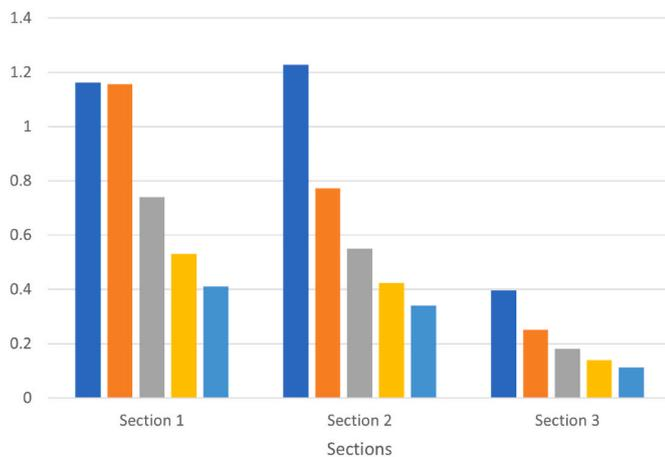
Fig. 2. Simulated fouling rate as a function of number of cycles. Five cycles were simulated with a flow of  $0.15 \text{ m}^3/\text{h}$  and a speed  $V = 0.53 \text{ m/s}$ .
