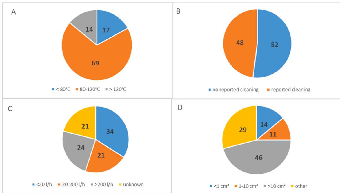
Fig. 5. General characteristics of the experimental setup to measure and study fouling behaviour in research recently reported in 32 articles. (a) Operating temperature, (b) Reported cleaning of the setup, (c) Capacity of the setup defined by product flow, (d) Area of surface at which fouling was measured.
