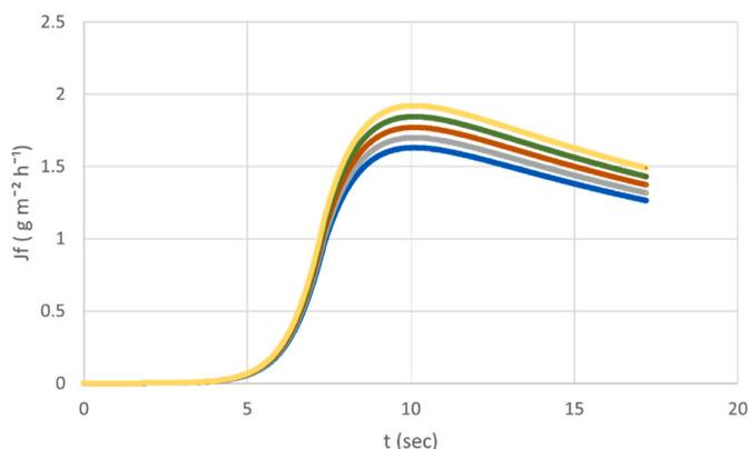
Fig. 3. Simulated fouling rates at the preheating ( $60\text{--}90^\circ\text{C}$ ) and the holding section ( $90^\circ\text{C}$ ) with different wall temperatures. The red line shows the fouling at  $90^\circ\text{C}$ . The two lower lines show the fouling with a change in wall temperature of respectively  $-1^\circ\text{C}$  and  $-2^\circ\text{C}$ , while the 2 top lines show the fouling with wall temperatures of respectively  $+1^\circ\text{C}$  and  $+2^\circ\text{C}$ .
